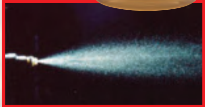
Injector spray pattern after P.i. treatment
