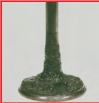
Intake valve before P.i. treatment
